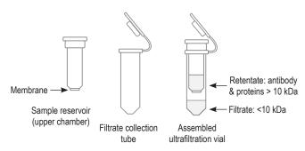
Figure 1. Ultrafiltration vial components.
